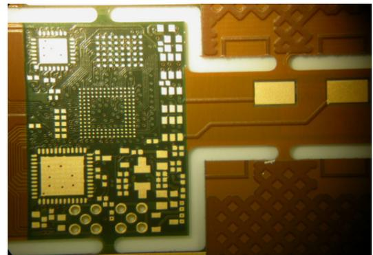
Flexible PCB of combined solder mask and coverlay type
