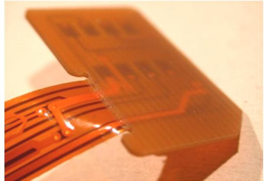
Flexible PCB with reinforcement
